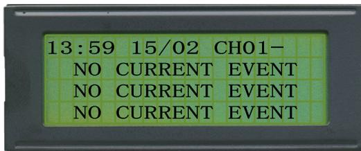
The example above shows that a Dial-out event occurred at 13:59 hours on the 15th of February and Channel 1 was the cause. The hyphen at the end means that there were no other active alarms.
