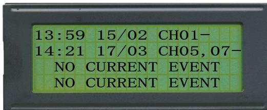
The example above shows that latest Dial-out event occurred at 14:21 hours on the 17th of March and Channel 5 and Channel 7 were the cause. The hyphen at the end means that there were no other active alarms.
