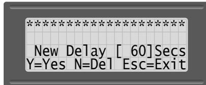
Enter the new Alarm delay in **SECONDS** (e.g. 60=1min, 600=10 minutes).
