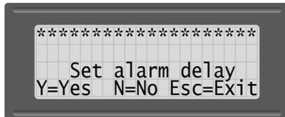
Press the 'Y' key to proceed in Editing the Alarm delay or the 'N' key to return to Keypad options.
