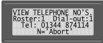
The 2<sup>nd</sup> Line on the display shows the current Roster selected and which telephone number you are viewing within the Roster.
