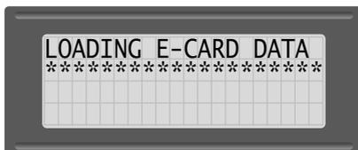
It will be noticed that a set of full stops travel from the left of the display towards the right, this is a visual indication that the data is being taken from your Config-Card and stored internally within the M60.
