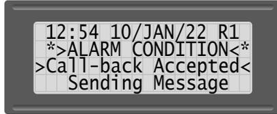
If no 'Call-back' is made the M60 will wait until the 'Call-back' period has elapsed and begin to telephone the next number in the 'Roster' sequence.
