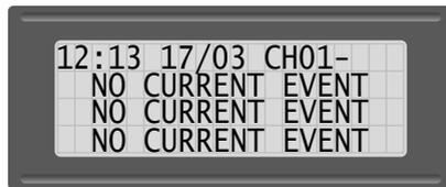
The example above shows that a Dial-out event occurred at 12:13 hours on the 17th of March, and Channel 1 was the cause. The hyphen at the end means that there were no other active alarms.
