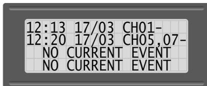
The example above shows that latest Dial-out event occurred at 12:20 hours on the 17th of March, and Channel 5 and Channel 7 were the cause. The hyphen at the end means that there were no other active alarms.
